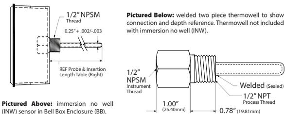
**Pictured Below:** welded two piece thermowell to show connection and depth reference. Thermowell not included with immersion no well (INW).
