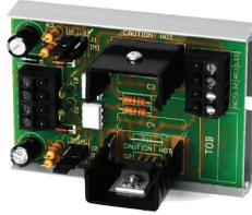
The TOB will accept up to two separate signals from up to two AC TRIAC outputs, or DC sources, and provide up to two TRIAC outputs each capable of driving a 2.5A load. Each output TRIAC is activated for the time that the signal is applied to the input. The TOB provides isolation between the input and output circuits as well as the two identical circuits.
