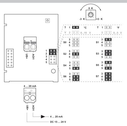
The adjustment of the measuring ranges is made by changing the bonding jumpers. The output value in the new measuring range is available after 2 seconds.
