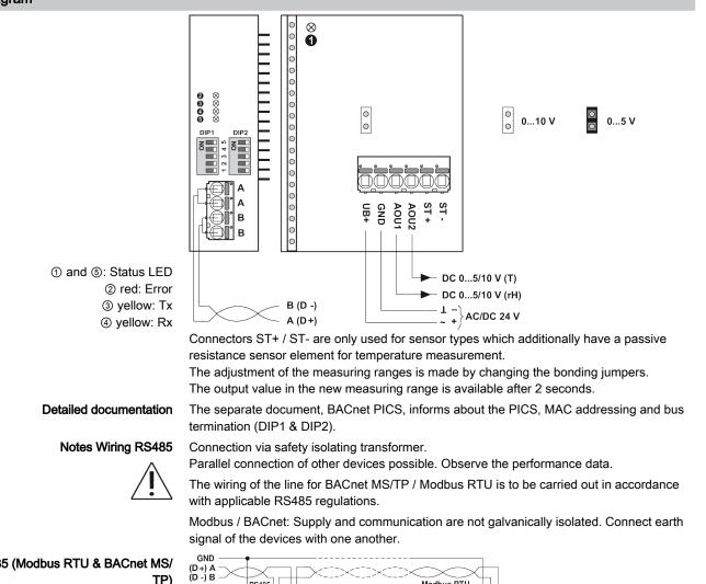
Wiring RS485 (Modbus RTU & BACnet MS/ TP) RS485
