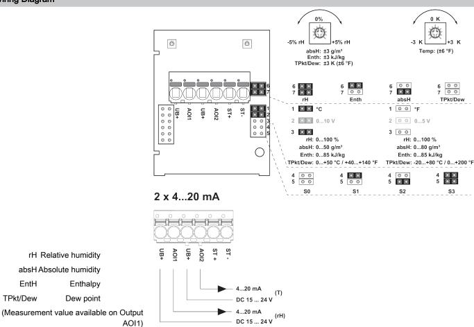
Connectors ST+ / ST- are only used for sensor types which additionally have a passive resistance sensor element for temperature measurement.
