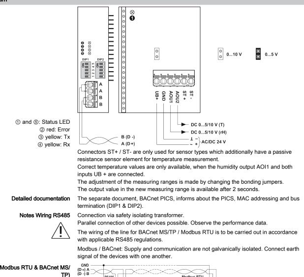
Wiring RS485 (Modbus RTU & BACnet MS/
