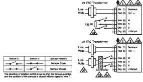
Multiple Actuators with Minimum Position Potentiometer
