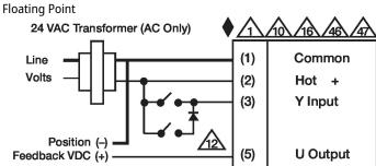
VDC/mA Control 24 VAC Transformer (1) Common Line Volts (2) Hot + 500 Ω 1/4 watt Control Signal (-) VDC/mA (+) (3) Y Input **Position** (5) **U** Output Feedback VDC
