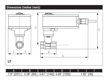
Modulating, Non-Spring Return, 24 V, for 2 to 10 VDC or 4...20 mA
