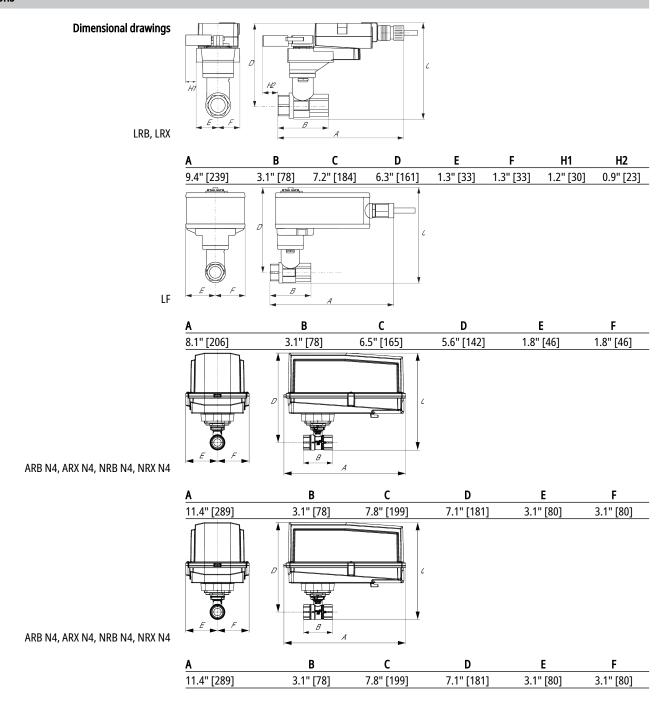
Modulating, Non-Spring Return, 24 V, 0 to 20 V **Phasecut**
