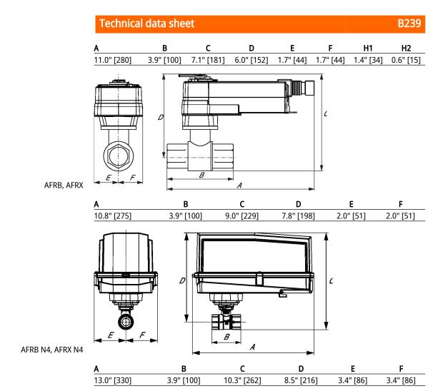
NEMA 4, Modulating Control, Non-Spring Return, Direct Coupled, 24 V, Multi-Function Technology®
