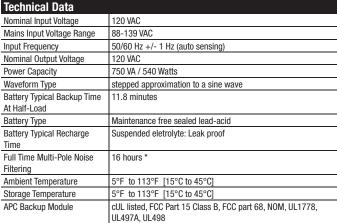
\*The time to recharge to 90% of full battery capacity following a discharge to shutdown using a loaded rated for 1/2 of the full load rating of the IIPS
