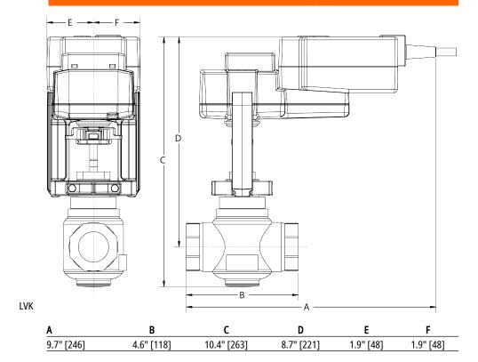
Modulating, Electronic Fail-Safe, Linear, 24 V
