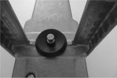
**3** Position the coupler support on the actuator spindle, with the indicators facing you.
