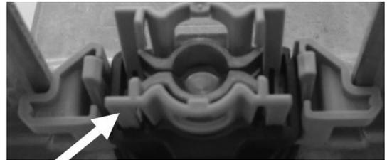
**7** Catch the clamps with the small ears of the clamp holder. Pinch the clamp holder together as shown. Catch the corners of the metal clamps by pushing down a bit on the clamp holder, so the ears are over the metal clamps. Do not force it or the plastic could break. If it does not grab all 4 corners take apart and do again.
