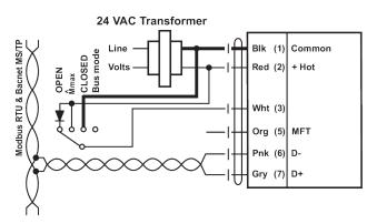
Modbus & BACnet control with local override (AC only, analog override) for Non-Spring Return
