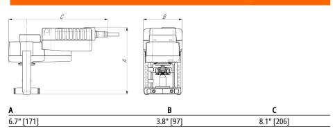
Modulating, Electronic Fail-Safe, Linear, 24 V
