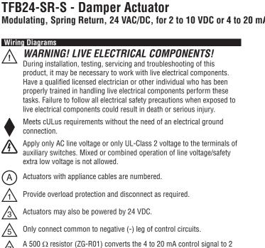
to 10 VDC. Actuators may be connected in parallel if not mechanically linked. Power /1\ consumption and input impedance must be observed.
