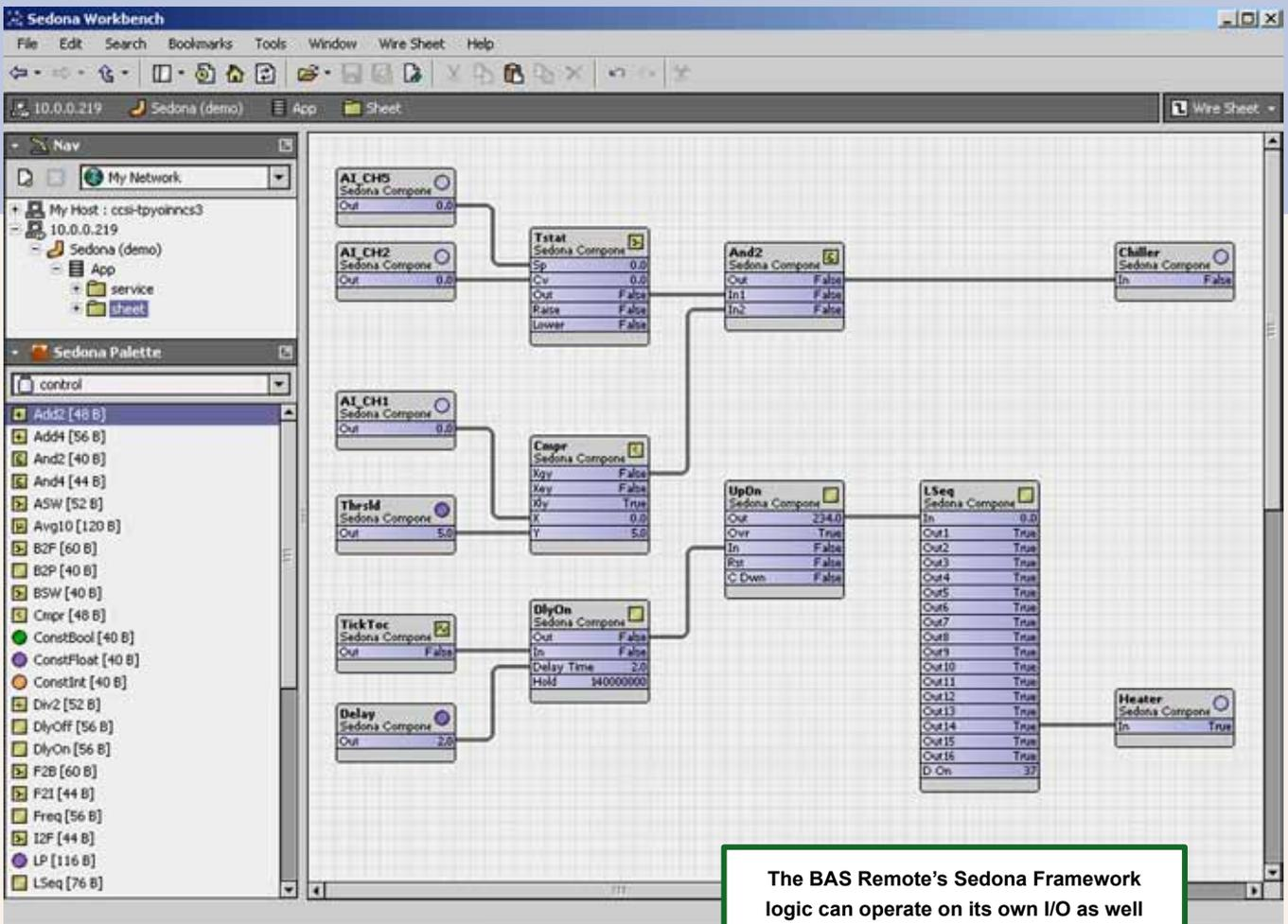
The BAS Remote's Sedona Framework logic can operate on its own I/O as well as that of connected Modbus serial devices. Also, a network connected Niagara Framework device can read or modify the operating state of the Sedona Framework function blocks.
