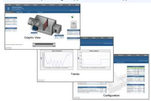
In the EC-Net<sup>AX</sup> solution, dc *gf*xApplications provide ready-to-use Px graphics pages for the ECB/ECL-VAV series of factory preloaded controllers. Once the controller is online, select any one of the standard VAV pre-configured controller applications to use. This provides a proven energy-efficient sequence of operation without any need for programming.
