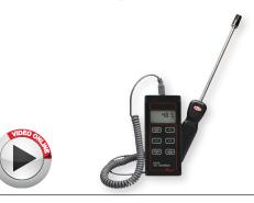
The Model 485B Thermo-Hygrometer is a versatile, compact, handheld instrument for measuring percentage of relative humidity and temperature in °F or °C. Dew point and wet bulb temperatures are derived from the relative humidity and temperature measurements and are displayed on the LCD.
