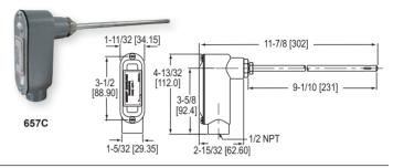
The Series 657 Relative Humidity/Temperature Transmitters provide two 4-20 mA channels to produce separate output signals for both relative humidity and temperature. These devices deliver  $\pm 2\%$  accuracy for humidity and  $\pm 1^{\circ}F$  for temperature measurements. Stainless steel probe can be easily mounted to most ductwork using either of the two optional kits below.
