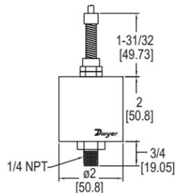
The **Series 682 Industrial Pressure Transmitter** is designed to withstand environmental effects such as shock, vibration, temperature, and EMI/RFI. The electronics and capacitive sensor are packaged in a welded stainless steel housing and meets NEMA 4 (IP65) protection ratings.
