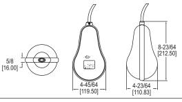
The Series FSW2 Free-Floating Level Switch is a self-counterweighted, mechanically actuated floating switch intended to activate electrical components, such as pumps, to start and stop automatically. Optional cables are available. Contact factory for cable length options ranging from 10 to 70' (3 to 21 m).
