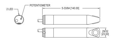
The Series AVFS Air Flow Switch is specifically designed to monitor air flow in ducts and provides a 3 A contact output to indicate a change or loss of flow. The AVFS provides a ±5% set point repeatability across a full-scale range of 1-10 m/s (197-1969 fpm) and includes a mounting bracket for quick duct mounting.
