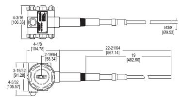
The Series CLS2 Capacitive Level Switch is a capacitive technology level switch which can be used for liquids, powders and bulk materials. It is offered with PVDF and 316 SS wetted material, weatherproof enclosure, DPDT output and a variety of process connections.
