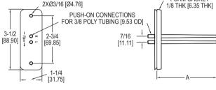
The Series PAFS-1000 Averaging Flow Sensors are ideal for sensing velocity pressure in the inlet section of variable air volume terminal units and fan terminal units.
