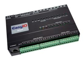
The EasyIO-30P controllers are rugged, network centric, multi-protocols Input / Output controllers to accommodate general and specific applications, featuring Bacnet IP, Bacnet Ethernet, Bacnet MSTP, Modbus Serial (RS485) and Modbus TCP/IP protocols. It also has a built-in web server for easy configuration.
