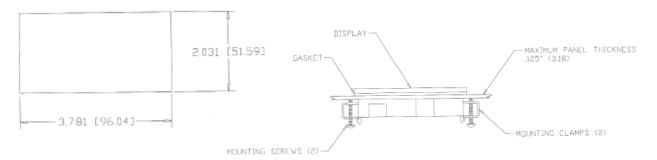
To install the BLL510 or BLV512 display module using the remote mounting kit (129-178-4 and -8):
