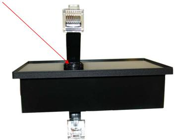
11. Plug the other end of the cable into the RJ45 style connector located on the BLL510/BLV512 display module.
