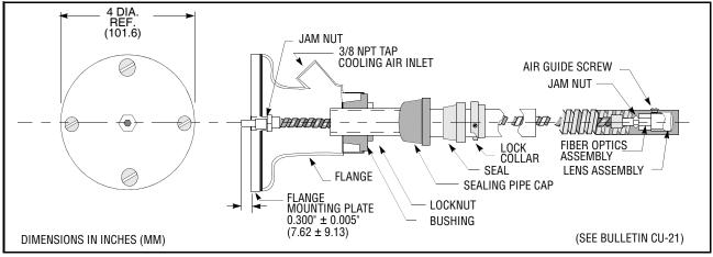
Following steps described in Bulletin CU-21, carefully remove the Inner Carrier Assembly's Flange Mounting Plate, Flange, Bushing and Locknut shown in Figure 4, above. Leave the original 1/4-28 Jam Nut on the Fiber Optic Bundle.
