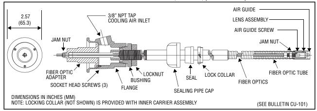
Following steps described in bulletin CU-101, carefully remove the quartz Inner Carrier Assembly's Jam Nut, (3) Socket Head Screws, Fiber Optic Adapter, Flange, Bushing and Locknut shown in Figure 3, above.
