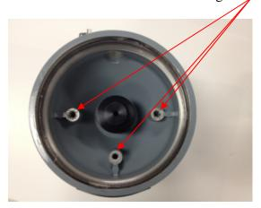
7. Position the new scanner electronics assembly into the CEX housing base.
