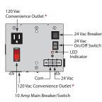
\* Move internal jumper to "HOT" position if you wish outlets to always be hot otherwise outlets will be switched by main breaker.
