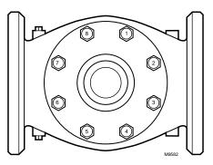
Fig. 3. Replacement V5055B/V5097B 4-inch valve bonnet assembly .
