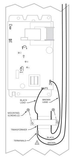
BROWN AND BLACK WIRES OFF OF P1 AND P2 TERMINALS CAN GO ON EITHER TRANSFORMER TERMINAL.
