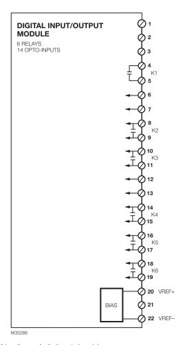
Fig. 3. Wiring diagram for limit control module.
