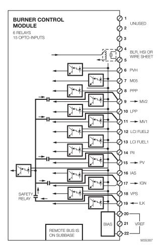
Fig. 3. Wiring diagram for Burner Control Module.
