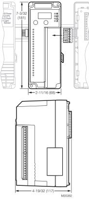
Fig. 1. Dimensions in in. (mm).
