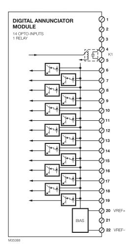
Fig. 4. Annunciator Module terminals.
