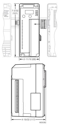
Fig. 1. Dimensions in in. (mm).
