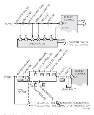
Fig. 3. Wiring diagram for Annunciator Module.
