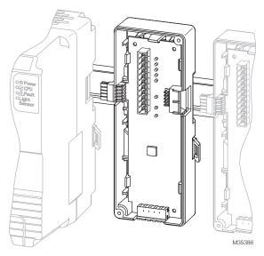
Fig. 4. Connecting additional sub-base modules.
