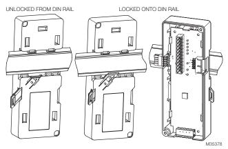
Fig. 3. Sub-base locking mechanisms.
