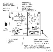
Fig. 1. Top view of standard capacity combination gas control.
