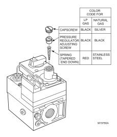
Fig. 2. Conversion kit installation.
