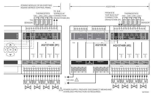
Fig. 9. Wiring of AQ25744B Expansion Zoning Panel to AQ2000 Series Control Panel.
