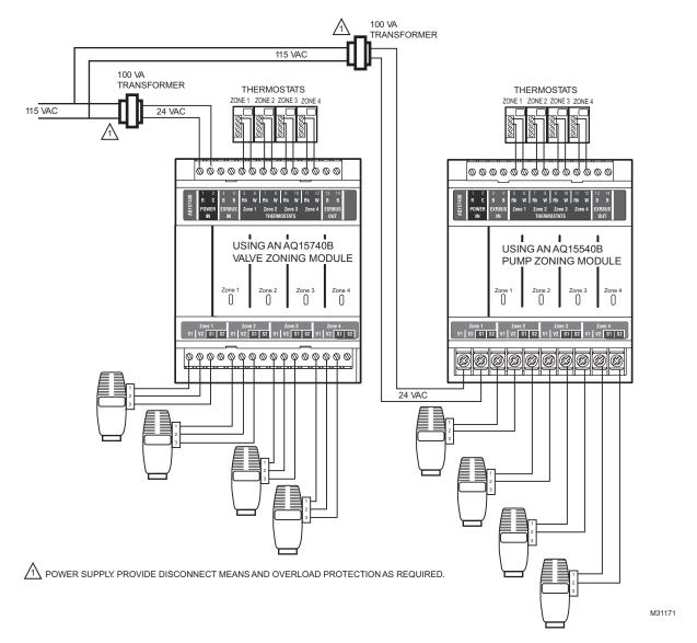
Fig. 7. Wiring of additional low voltage VA capacity.
