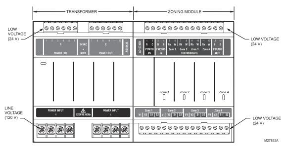
Fig. 2. AQ257 Expansion Zoning Panel Layout (AQ25744B shown).
