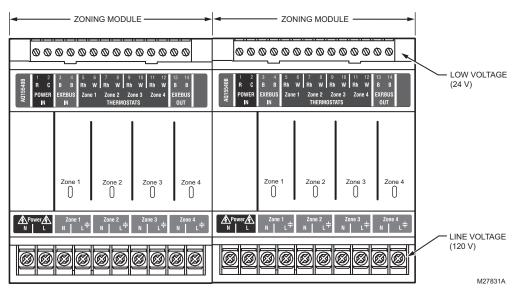
Fig. 1. AQ255 Expansion Zoning Panel Layout (AQ25582B shown).
