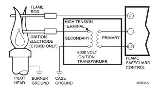
Fig. 6. Typical field wiring diagram for C7005 gas pilot and flame rod assembly.
