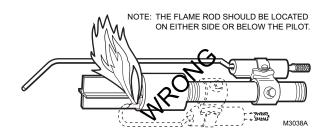
Fig. 2. Improper position of flame rod assembly in in. (mm).
