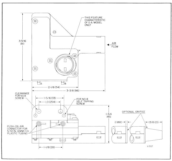
Fig. 1. Approximate Sensor Dimensions in Inches (mm).
