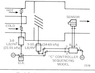
Fig. 5. Dual Duct Variable Constant Volume Application.
