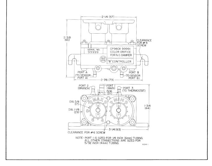
Fig. 2. Approximate Controller Dimenions in Inches (mm).
