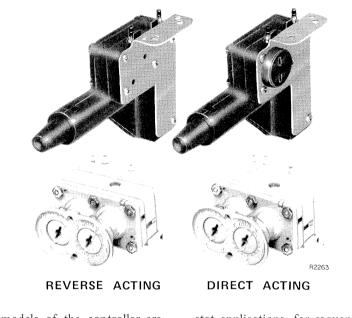
Two models of the controller are available. A type "B" controller provides high and low air volume limits and is used in conjunction with a 1-pipe bleed thermostat. A type "C" controller is used for two-pipe thermostat applications, for sequencing with reheat, and in certain dual duct applications. Both "B" and "C" controllers can be reverse or direct acting (corresponding to R.A. or D.A. sensor).
