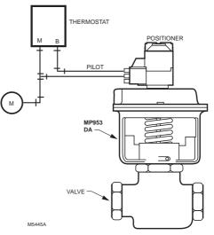
Actuator Type: Valve Temperature Range: 0 F to 140 F (-18 C to +60 C) Maximum Operating Pressure: 25 psi (172 kPa) Humidity Range: 5 to 95% RH
