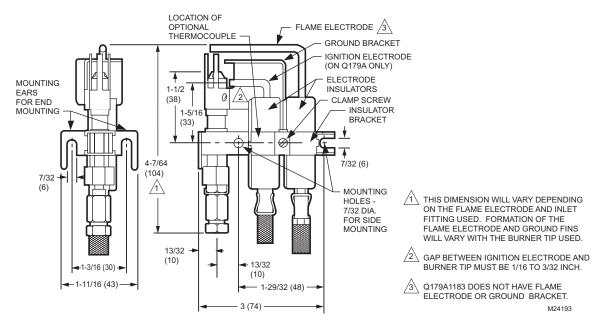
Fig. 2. Approximate mounting dimensions in inches. (mm) and arrangement of parts.
