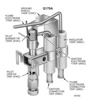
Fig. 3. Component maximum temperature ratings. (Q179A1126 model shown)
