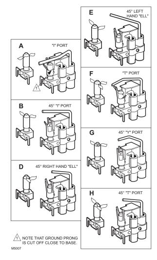
Fig. 1. Pilot tip assembly styles.
