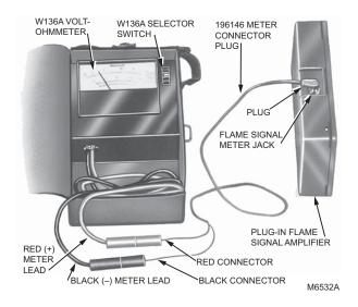
Fig. 4. Measuring microamp flame signal.
