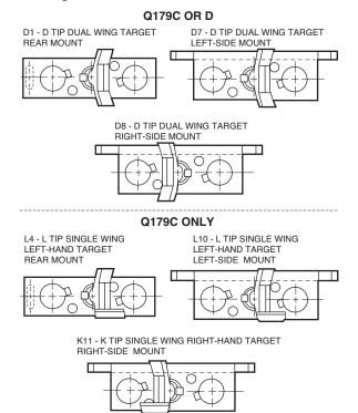
NOTE: MOUNTING NUMBER DESIGNATES BOTH BRACKET TYPE AND TARGET CONFIGURATION. DESCRIPTION REFERENCE POINT IS FROM BACK OF BURNER TARGET. M3054A
