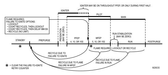
Fig. 23. Interrupted pilot.
