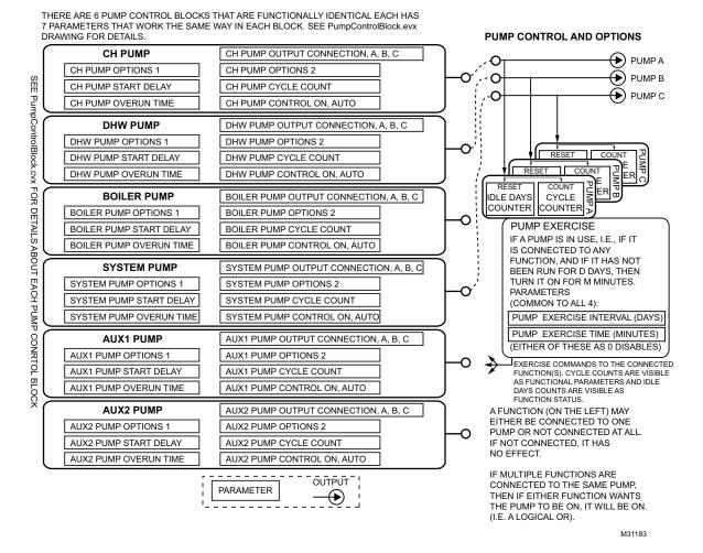
Fig. 21. Pump control blocks.
