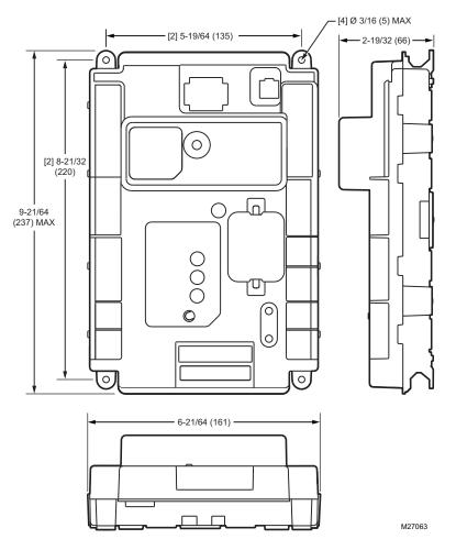
Fig. 2. R7910A/R7911 dimensions in in. (mm).
