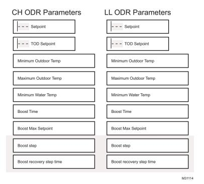
Fig. 10. Outdoor reset parameters.
