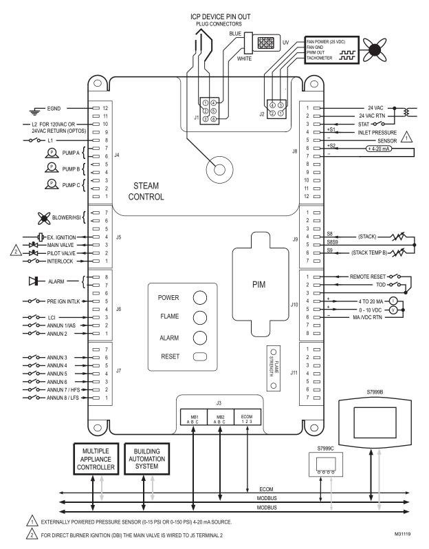
Fig. 4. R7911 device pin out.
