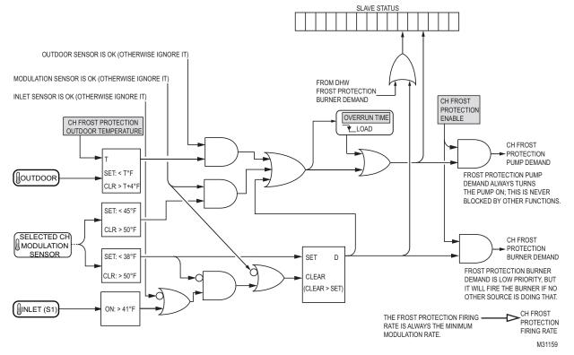
Fig. 17. CH Frost protection.
