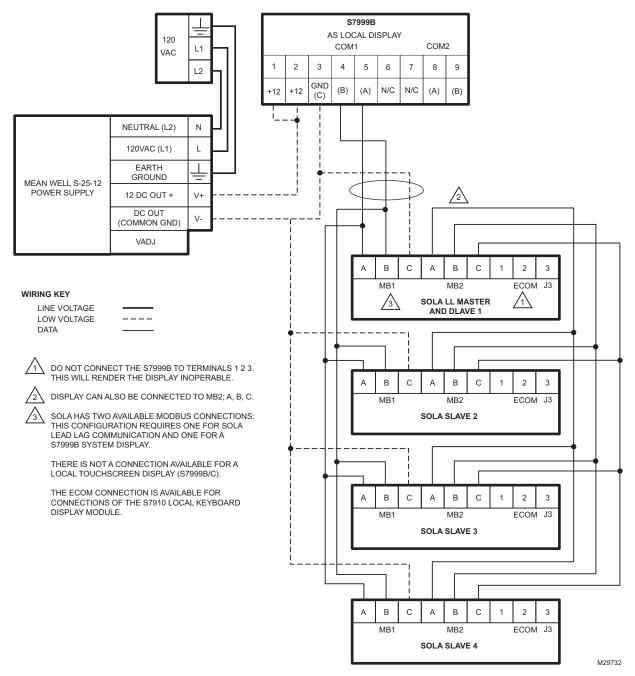
Fig. 28. S7999B system and lead lag wiring diagram.
