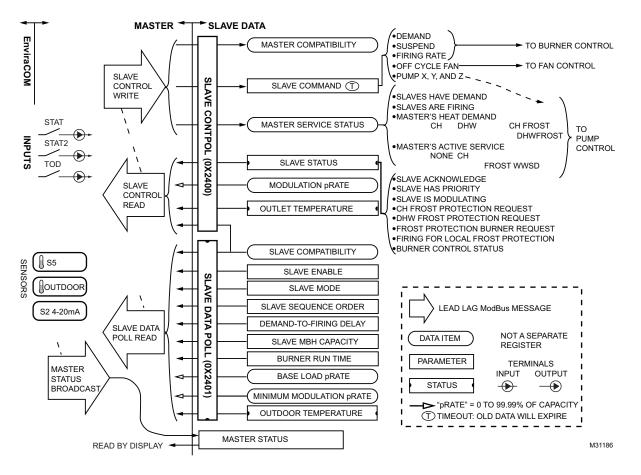
Fig. 29. Master/Slave data transmission.
