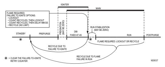
Fig. 25. Direct burner ignition
