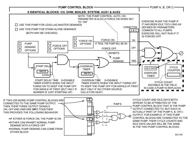
Fig. 22. Pump control block.
