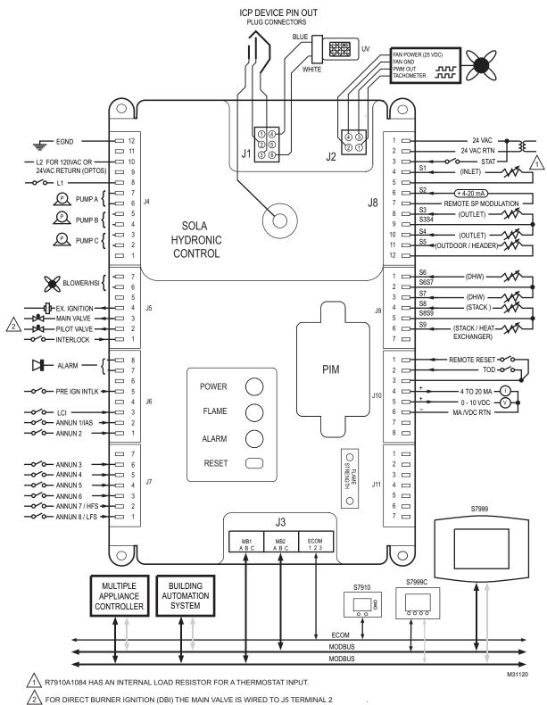
Fig. 3. R7910A device pin out.
