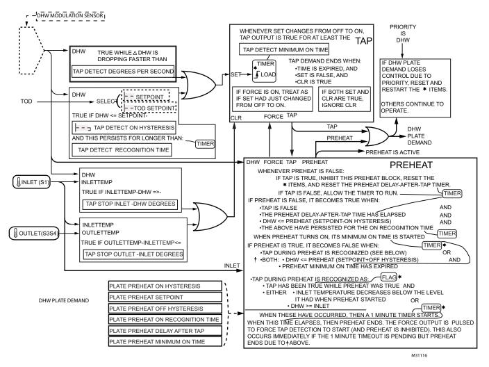
Fig. 15. Plate heat exchanger subsystem.
