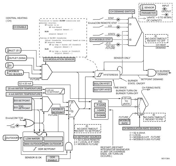
Fig. 8. Central heating hydronic diagram.
