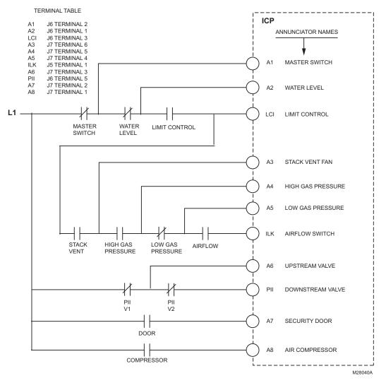
Fig. 26. Example of annunciator inputs and terminal names.
