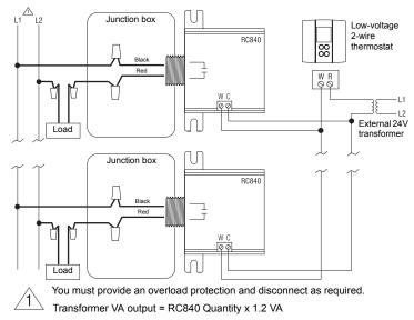
Figure 3 : Connection to a 2-wire low voltage thermostat using a 24 V external transformer and multiple relays
