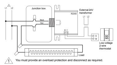
Figure 1 : Connection to a 2-wire low voltage thermostat using a 24 V external transformer
