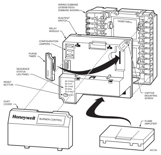
Fig. 4. RM7845A Relay Module exploded view.
