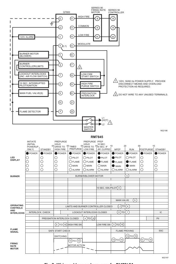
Fig. 3. Wiring subbase and sequence for RM7845A.
