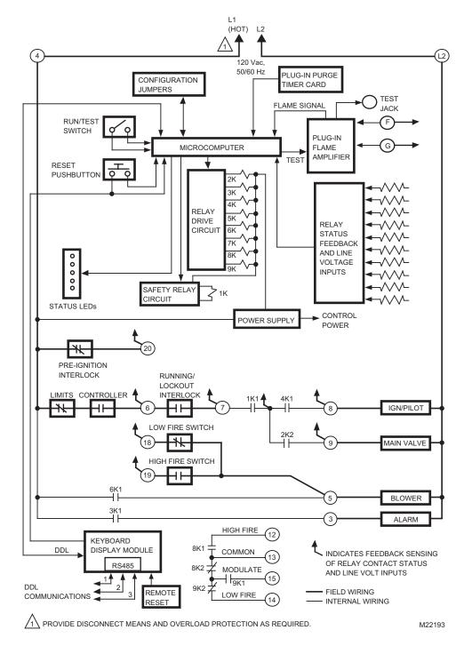
Fig. 2. Internal block diagram of the RM7845A (See Fig. 3 for individual detailed wiring instructions).
