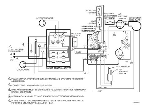
Fig. 9. SV9410/SV9420; SV9510/SV9520; SV9610/SV9620 typical boiler wiring diagram.
