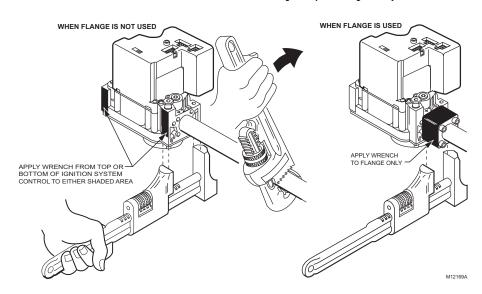
Fig. 5. Proper use of wrench on ignition system control with and without flanges.
