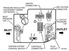
Fig. 4. Top view of ignition system control.
