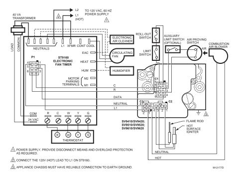
Fig. 7. SV9410/SV9420; SV9510/SV9520; SV9610/SV9620 typical wiring connections in fan-assisted warm air furnace with ST9160 Fan Board.
