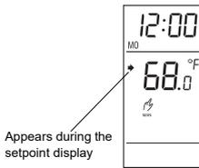
To adjust the setpoint, press one of the  $\blacktriangledown$   $\blacktriangle$  buttons until the desired temperature is displayed.
