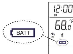
The time and programming are saved for the first 15 seconds when the batteries are removed.
