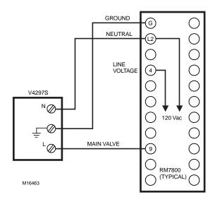
Fig. 5. Typical wiring diagram for V4297 NOVV.
