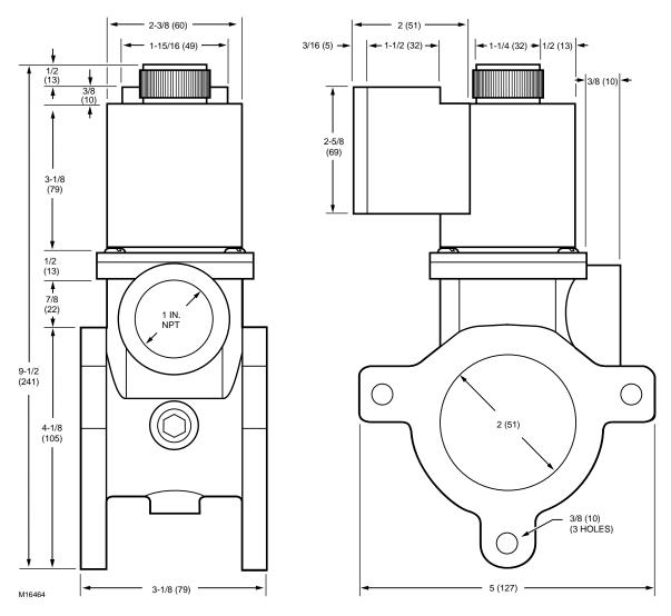
Fig. 2. Approximate dimensions of smaller V4297 NOVV in in. (mm).
